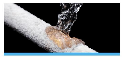
When water-filled systems freeze, the formation of ice can result in obstructions, impaired water flow and malfunction of systems. A freeze-up is usually first identified by a loss of water pressure or flow. For fire protection systems, the freeze-up may represent a hidden threat that is not immediately apparent. Since water expands when it freezes, if it occurs within piping systems, it can eventually lead to broken pipes, valves and fittings.
